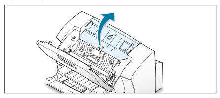
5. Locate the color and black print cartridge holders inside the machine.
